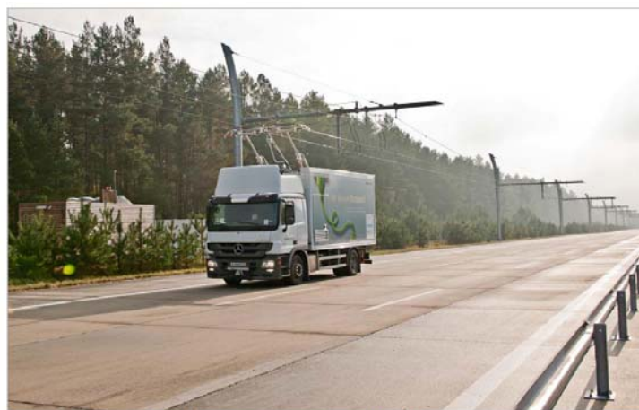
Siemens catenary hybrid truck in operation (source: Siemens Mobility)
